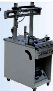
Handling sorting station
